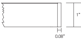
Ref Group TE HPL laminate over a 1” MDF core with matching or solid PVC edge.
