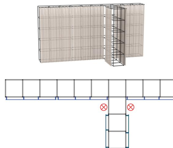
**X** Rule: When using curtain on the inner face one bay needs to be kept clear when another frame is running perpendicular
