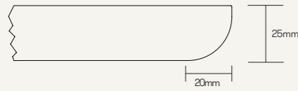
Ref Group Number 46 25mm MDF core, specified laminate face & counterbalance with 20mm chamfered edge. The edge is clear finish as standard or can be stained.
